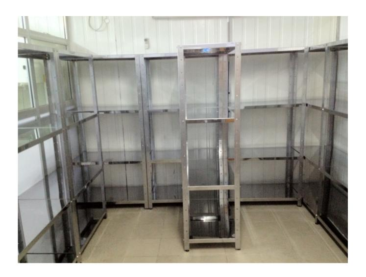
This form of shelving is widely used in both the industrial and commercial environment such as cold rooms and storage of oxidizing compounds. The components are robust and the shelves can carry up to 160kg's per shelf level. Stainless steel shelves are from 1.2mm grade 430 Stainless steel on uprights from 2mm all in brushed finish.
